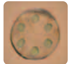
Cross section picture for RENCON 130
